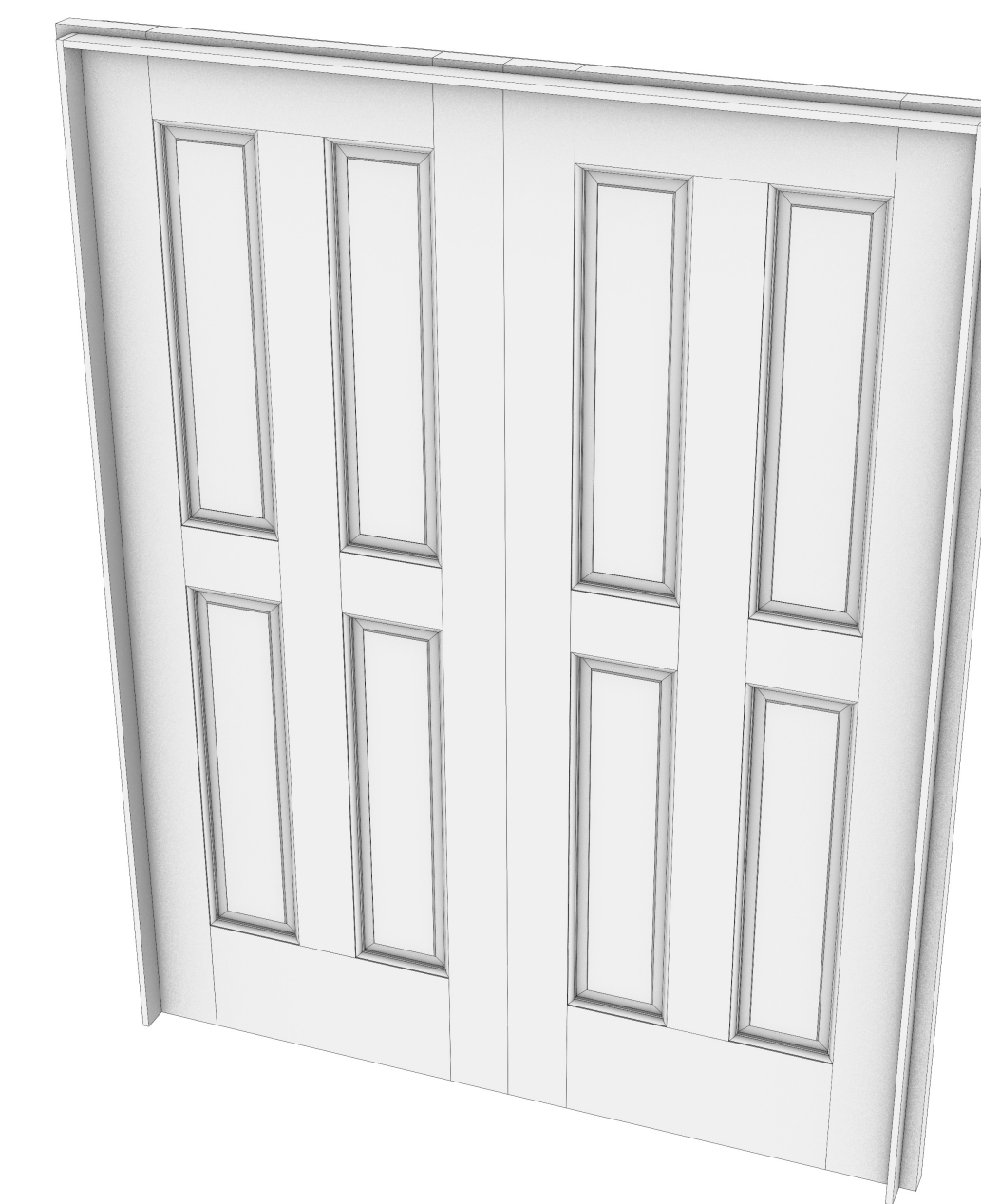
D5 DOOR #5: DOUBLE POCKET, 5'-1" FULL SCALE
